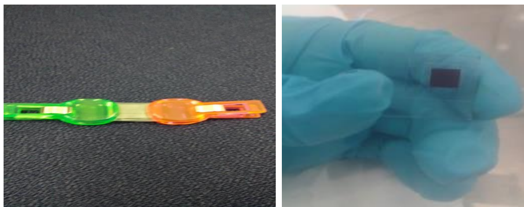
Fig.1. Photograph of assemble EDLC and DSSC using maximum conducting ILDPE.
